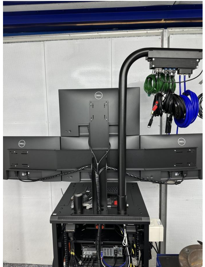
Rear view – cables routed down the bracket post to the PC
